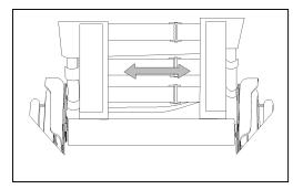
For V500 Light 30° with toothed adjustment: when the backrest is adjusted to the lowest position, the bottom strap can not be used. Remove the strap from the frame tubes by loosening the velcro.
