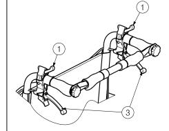
If your wheelchair features drum brakes, the handles 3 are used as brakes.
