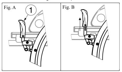
To apply the brakes (Fig A):
